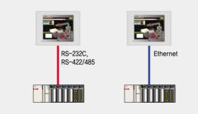
$\ast \text{Cress}$  cable is needed for the Ethernet 1:1 communication
