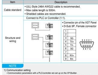
· Refer to the communication user manual about the communication wiring with a PLC/controller. · Set up a terminal resistance using a dip switch.
